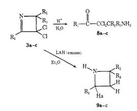
no other products present. The structures of azetidines 9a-c were obvious from their ir, nmr, and mass spectra. That the geminal hydrogens were in the 3 position in **9a** and **b** was indicated by the low-field ( $\tau$  5.4) broad triplet for H<sub>a</sub>. In 9c H<sub>a</sub> could not be resolved, but the mass spectra showed the expected  $\alpha$  cleavage at m/e 43 (CH<sub>3</sub>CH==NH·+) and no peak at m/e 30  $(CH_2 = NH \cdot +).$
